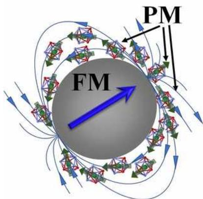
Fig. 1. Model of a composite material based on PrDyFeCoB microparticles (MP) and Er<sup>3+</sup> complex (PM). The internal field of particles is indicated by an arrow. The Er<sup>3+</sup> complex is located in the region of the stray field of microparticles.
