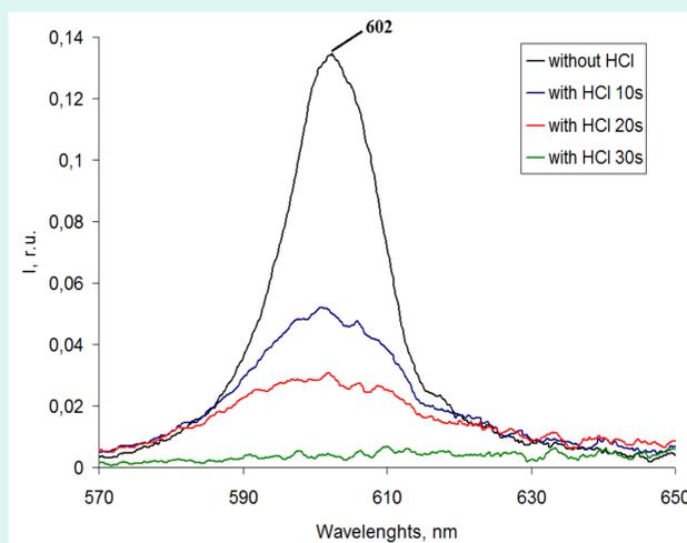
Fig.4. Lasing spectra of a PMMA film from a solution of tetrahydrofuran doped with NR with HCl vapor
