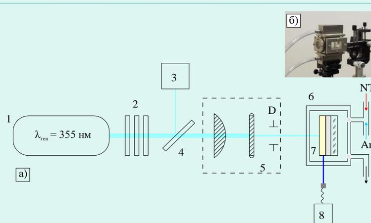
Fig. 3. (a) Scheme of the setup for measuring the spectral-luminescent and lasing characteristics and (b) gas cell photograph: ( 1 ) Nd<sup>3+</sup> : YAG laser ( $\lambda = 532$  nm); ( 2 ) system of non-selective light filters; ( 3 ) Gentec EO ED-100A-UV energy meter; ( 4 ) beam splitter; ( 5 ) pump beamforming optical system; ( 6 ) gas cell; ( 7 ) thin-film sample under study; ( 8 ) AvaSpec-2048 spectrometer; (b) photo of sealed cuvette.
