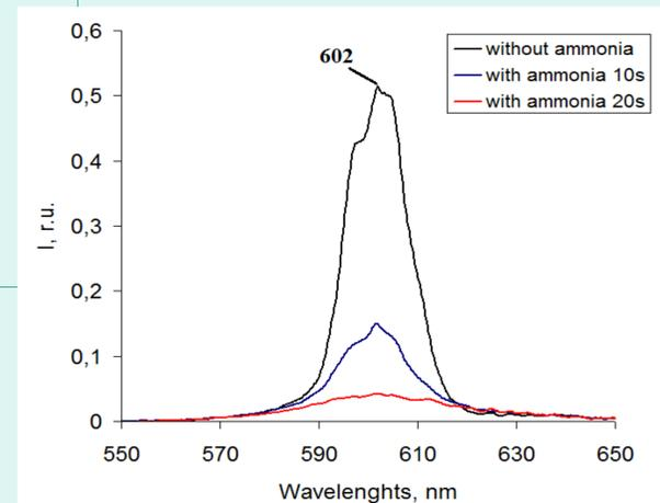
Fig.5. Lasing spectra of a PMMA film from a solution of toluene doped with NR with NH<sub>3</sub> vapor
