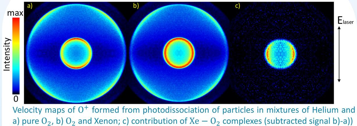
Velocity maps of  $\text{O}^+$  formed from photodissociation of particles in mixtures of Helium and a) pure  $\text{O}_2$ , b)  $\text{O}_2$  and Xenon; c) contribution of  $\text{Xe} - \text{O}_2$  complexes (subtracted signal b-a)
