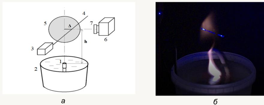
Fig.2. a) Scheme of observations of aerosol scattering in a laser beam. 1 - central electrode, 2 - discharge cell, 3 - laser, 4 - laser beam or vertical "laser knife", 5 - plasmoid, 6 - high-speed video camera, 7 - objective lens with focal length of 105 mm or horizontal microscope. b) Observation of aerosol in scattered light of the laser beam at the moment of plasmoid extinguishing.
