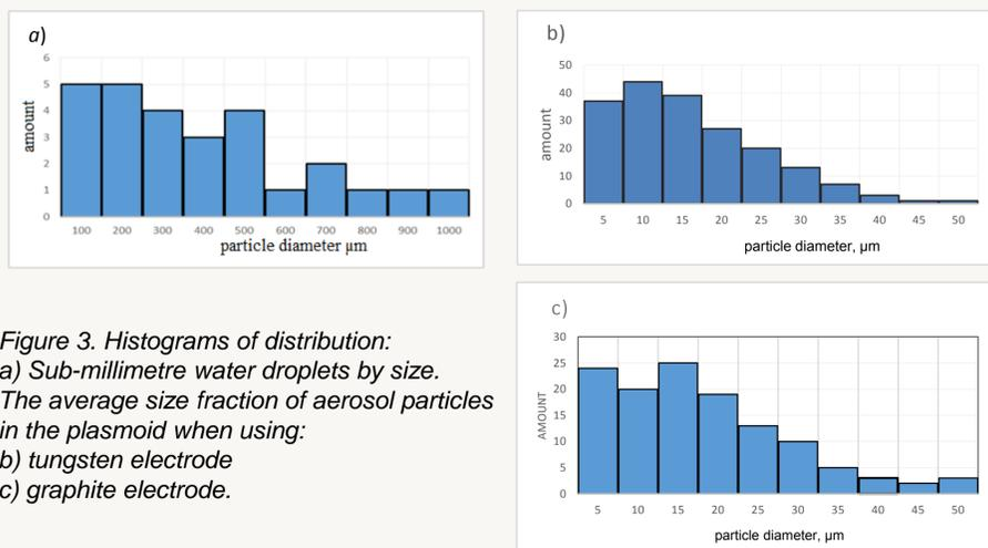
Figure 3. Histograms of distribution: a) Sub-millimeter water droplets by size. The average size fraction of aerosol particles in the plasmoid when using: b) tungsten electrode c) graphite electrode.
