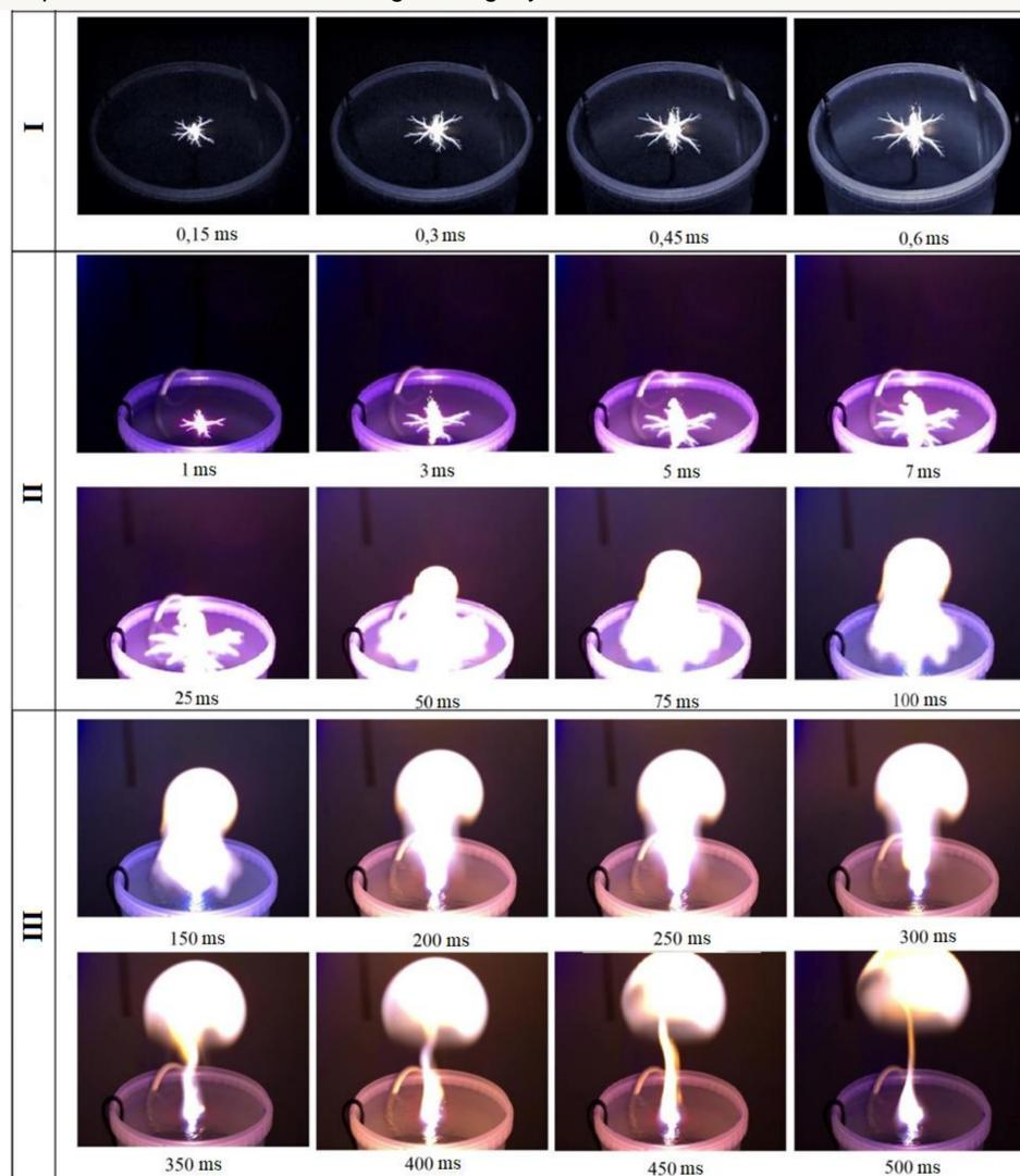
Fig. 4. Evolution of a plasmoid. Shooting parameters: (top row) shooting frequency 6400 fps, frame exposure time 60 μs; (remaining frames) shooting frequency 3200 fps, exposure time 100 μs.
