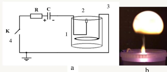
Fig. 1. a) Electrical scheme of the installation. b) Photo of the plasmoid. 1 - discharge cell, 2 - connection of central electrode located above water surface, 3 - second electrode submerged into water, 4 - key K; C - battery of high voltage capacitors, R-resistance limiting discharge current.
