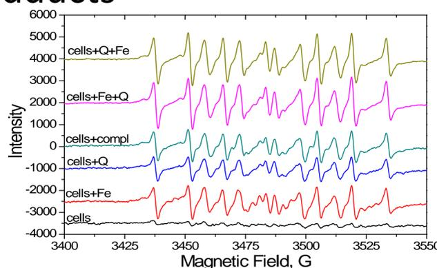
EPR spectra of solutions of cells MOLT-4 (1 ml/ml) with spin trap DEPMPPO (10<sup>-1</sup> M) in buffer HEPES (50mM) and NaCl (150 mM) (pH 7.1) with 1% DMSO; Q1 (50 mcM); Fe(NO<sub>3</sub>)<sub>3</sub> (50 mcM); [Fe(Q1)<sub>3</sub>] (40 mcM).
