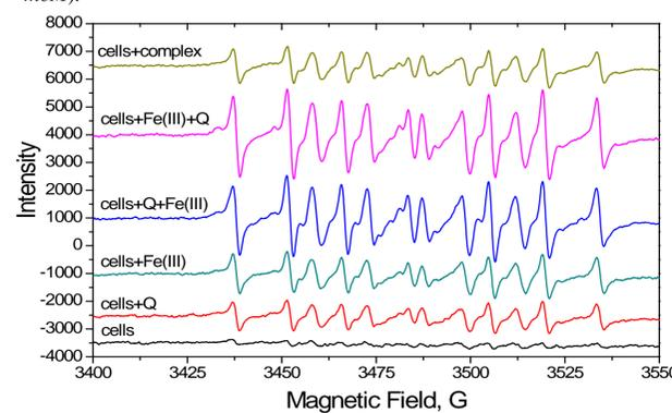
EPR spectra of solutions of cells A549 (1 ml/ml) with spin trap DEPMPPO (10<sup>-1</sup> M) in buffer HEPES (50mM) and NaCl (150 mM) (pH 7.1) with 1% DMSO; Q1 (50 mcM); Fe(NO<sub>3</sub>)<sub>3</sub> (50 mcM); [Fe(Q1)<sub>3</sub>] (40 mcM).
