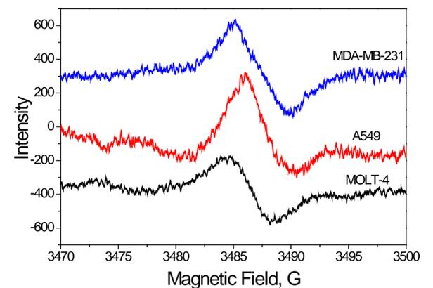
EPR spectra of cell cultures MOLT-4 (black), A549 (red), MDA-MB-231 (blue) (1 ml/ml) in HEPES buffer (50 mM) with NaCl (150 mM) (pH 7.1) with 1% DMSO in presence Q1 (50 mcM/L).
