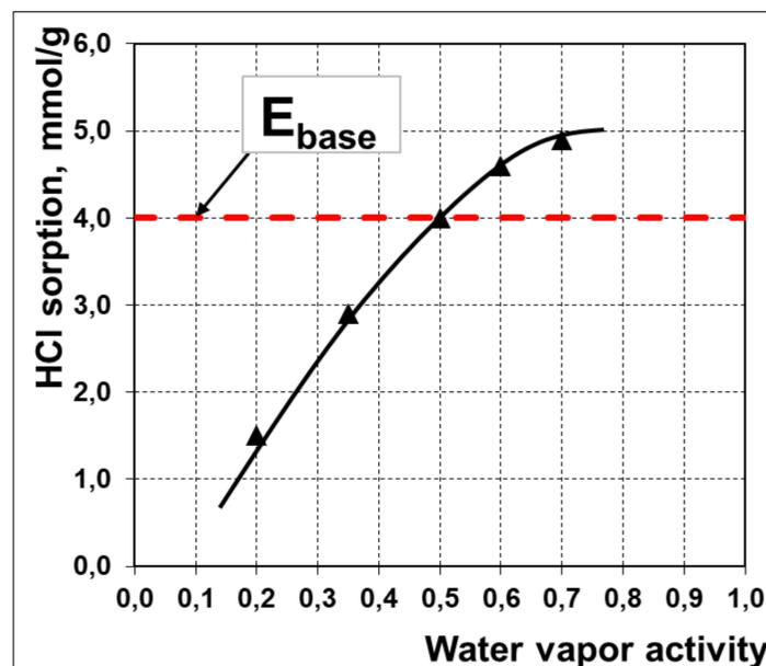
Fig.1 Sorption of HCl by ion exchanger PAN-EDA as a function of relative air humidity. Experimental conditions: temperature 20-22°C; thickness of the filtering layer 9-10 mm; air flow velocity through the filtering layer 0,1m/s; initial HCl concentration 55-57 mg/m<sup>3</sup>.
