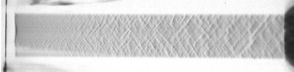
High-speed streak camera. The glow of the detonation front in the mixture of NM/NB 66/34.
