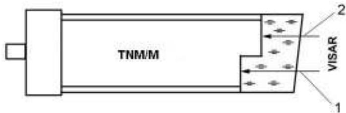
The scheme of the experiment when registering velocity profiles in two sections of the studied explosive.
