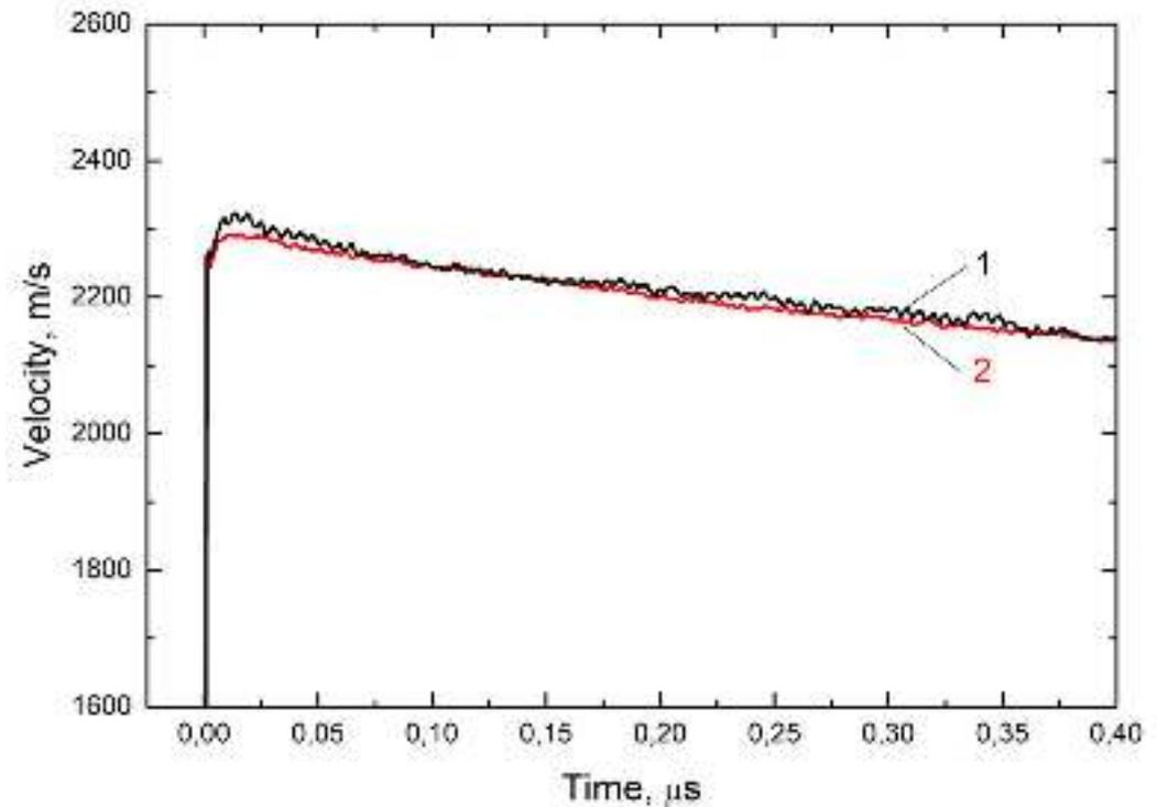
Velocity profiles at the boundary of the mixture TNM/M 85/15 with water in two different sections of the explosive
