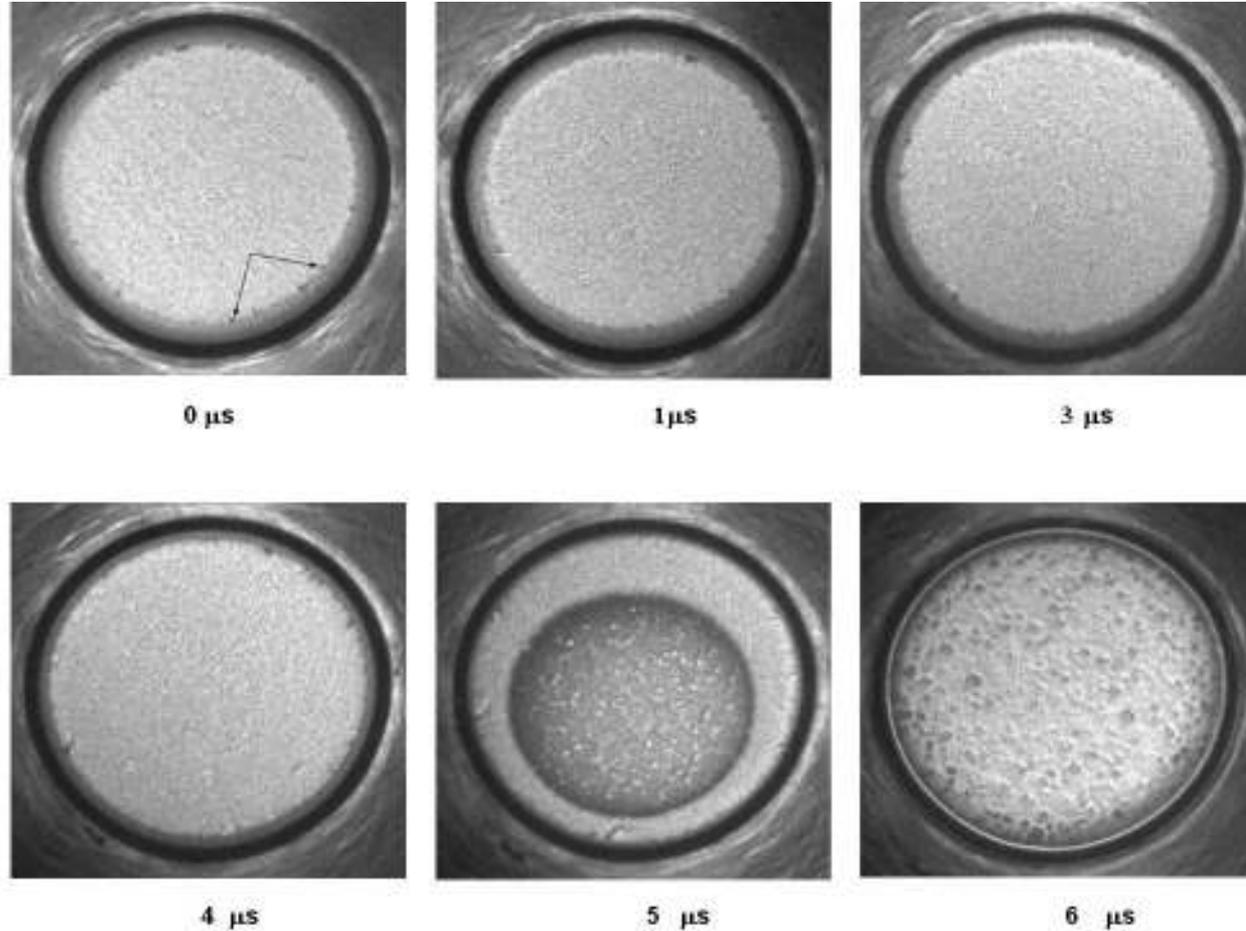
**NANOGATE-22/16 High-Speed Camera. The glow of the detonation front in the mixture of TNM/M 50/50.**
