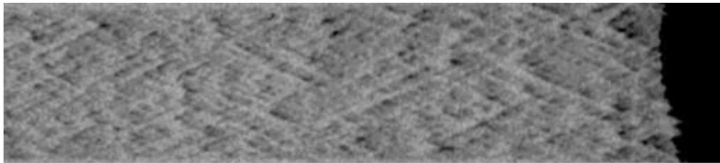
High-speed streak camera. The glow of the detonation front in the mixture of NM/M 65/35.
