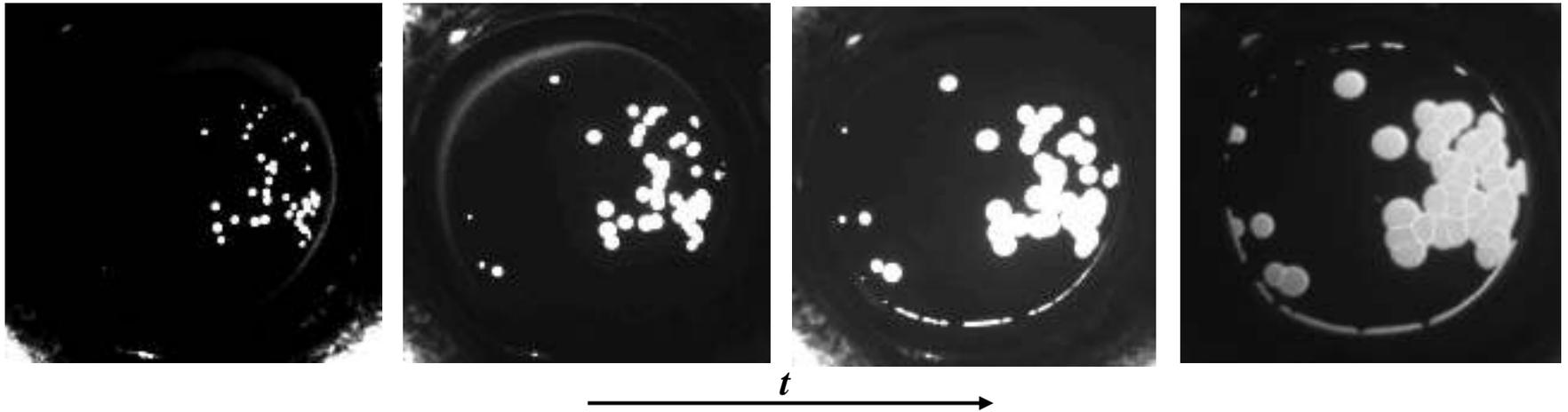
NANOGATE-22/16 High-Speed Camera. The glow of the detonation front for TNM/NB. The interval between frames is 0.1 microseconds
