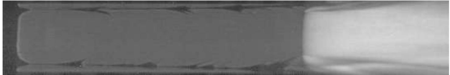
High-speed streak camera. The glow of the detonation front in NM.
