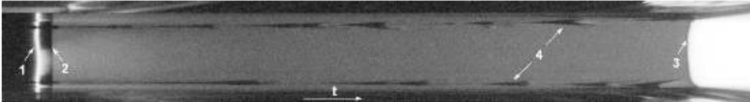
High-speed streak camera. The glow of the detonation front in the mixture TNM/NB 35/65
