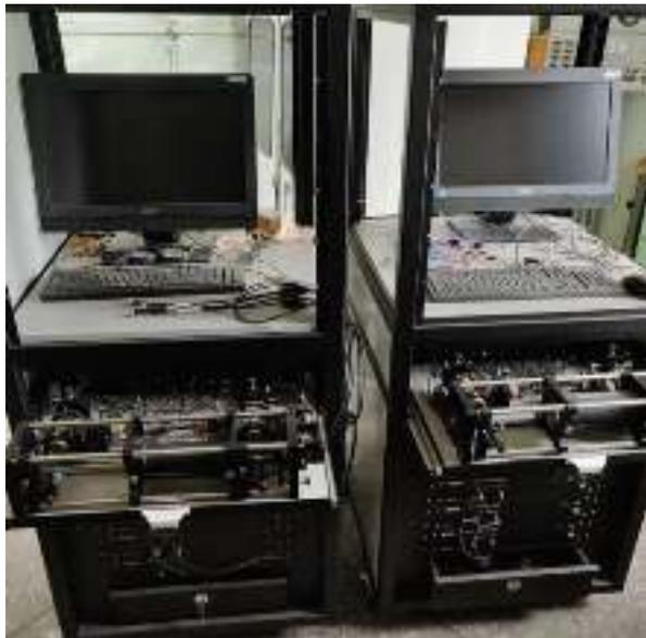
8-channel laser interferometer VISAR
