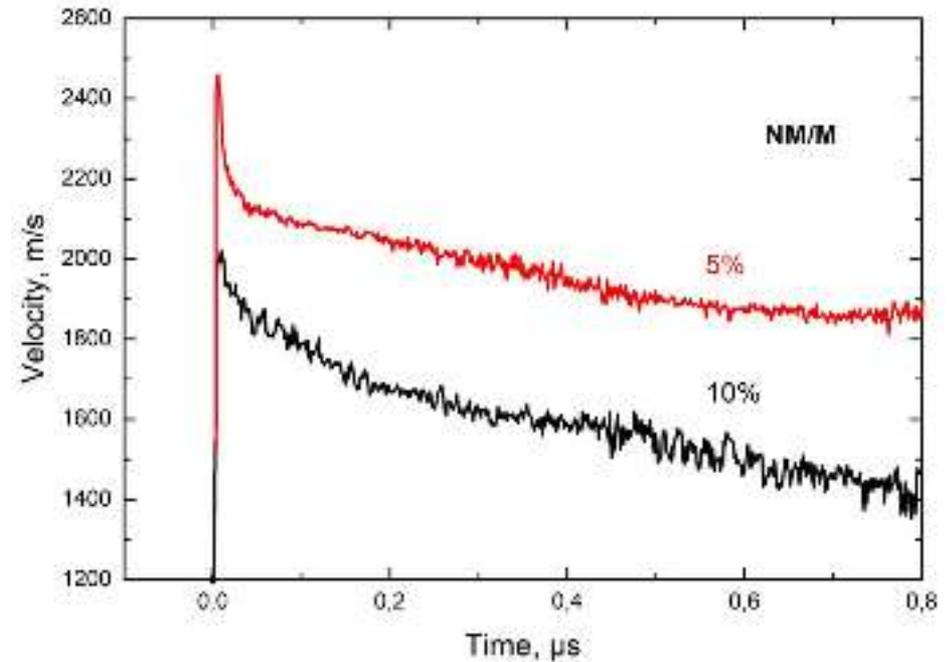
Velocity profiles of the mixture NM/M at the water boundary
