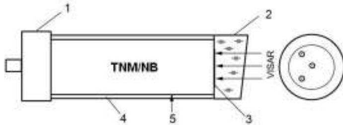
1 – plane shock wave generator; 2 – water window;
