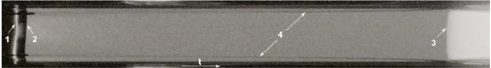
High-speed streak camera. The glow of the detonation front in the mixture TNM/M 60/40.
